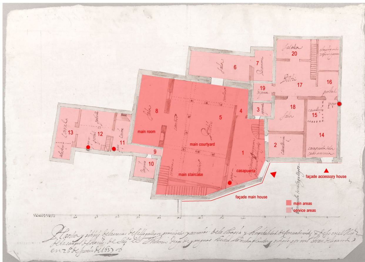
Fig. 16 Floor plan with indications of access points and areas of the house and the route according to the survey (Source: Hospital de las Cinco Llagas Collection, ADPSE, Seville, Spain and the authors)
