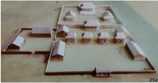
Figure 25 Wind erosion experiment on 1:500-scaled model (Source: Xiaoyu Wang).
