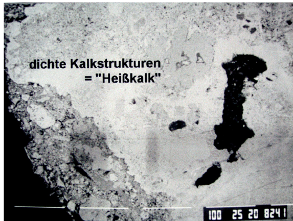
Fig. 16 Bratislava, castle, wall painting fragment of Regnum Maravorum (B1), 2nd half of the ninth century; favored by 'dry-slaking' (i.e. the mixture of non-washed sand and fresh lime before slaking), the fine silicates cause hydraulic reactions; analysis Hubert Paschinger, Federal Heritage Office, Vienna, No. 1240/98 (Source: Hammer 2008,122)
