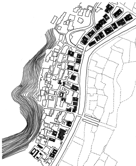
Fig. 3 Overall site layout, with a series of surgery-like renovations and adaptations in the central and southern parts of the village and a new residential area to the north that is composed of a newly planned street, 24 houses and a wind-rain bridge (Source: the author)
